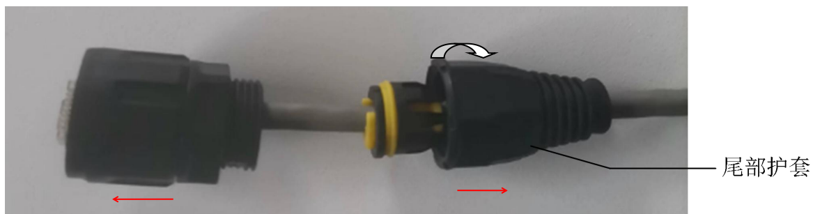
Figure 4-7 Communication cable threading
